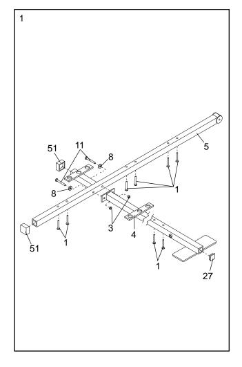
Slide the Assist Upright (74) and the Leg Press Upright (56) onto the indicated 5/16" x 2 1/2" Carriage Bolts (1) in the Stabilizer (5). The high side of the brackets on the Assist Upright and Leg Press Upright should be on the side shown. Hand-tighten four 5/16" Nylon Locknuts (3) onto the Carriage Bolts. Do not tighten the Nylon Locknuts yet.
